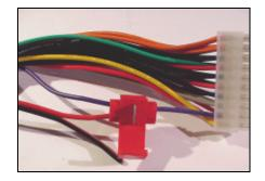
You put the clamp around the purple wire, lead the end of the wire that is to be connected into the opening and then you turn the latch down. Shut the clamp firmly. (It goes very heavily - perhaps use a pliers)
